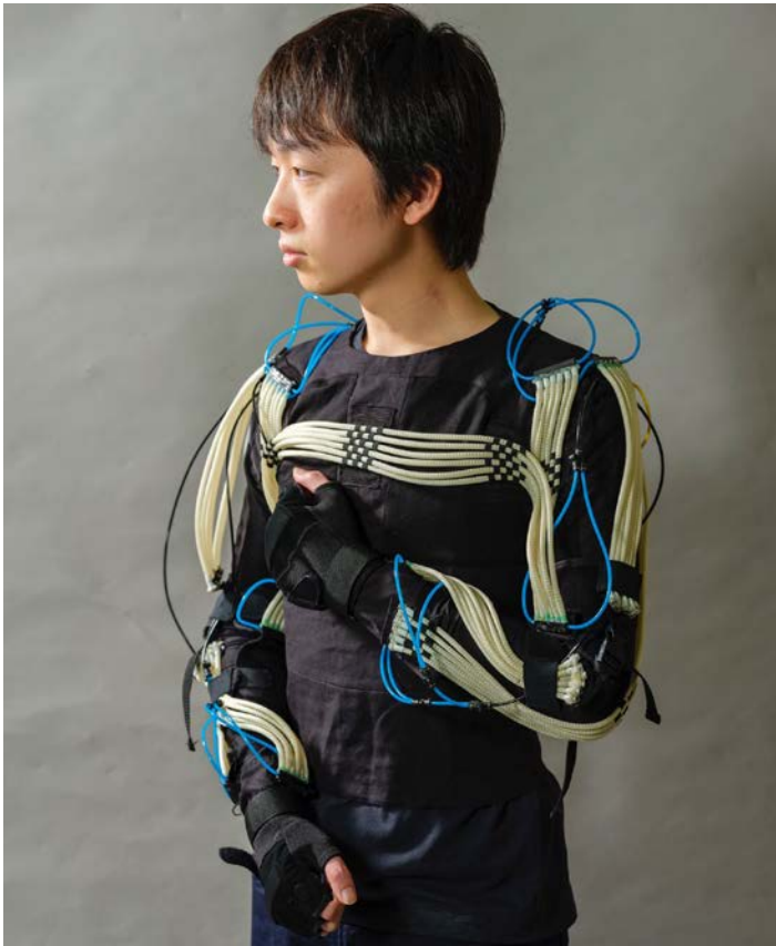
Abe T, et al. IEEE Robotics and Automation Letters. 2019 S-muscle (Suzumori, Tokyo Tech)
