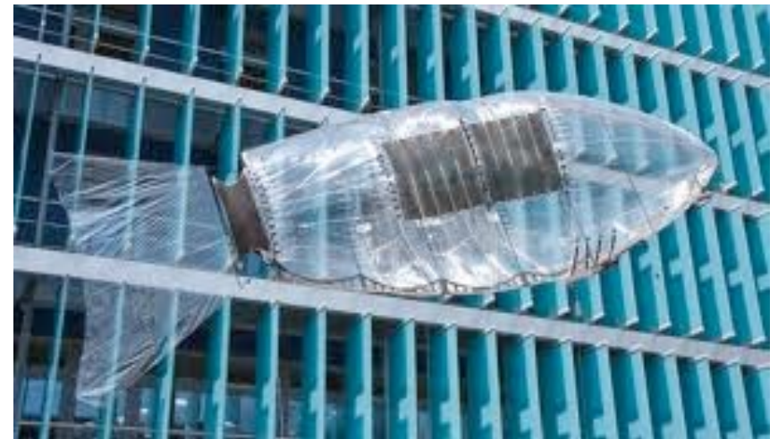
EMPA's (Zurich) 7 m long blimp: "swims" through the air using 4 artificial muscles
