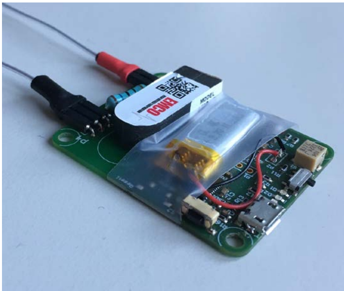
Miniature 1 channel 5 kV 1 Hz power supply: 16.0 g
